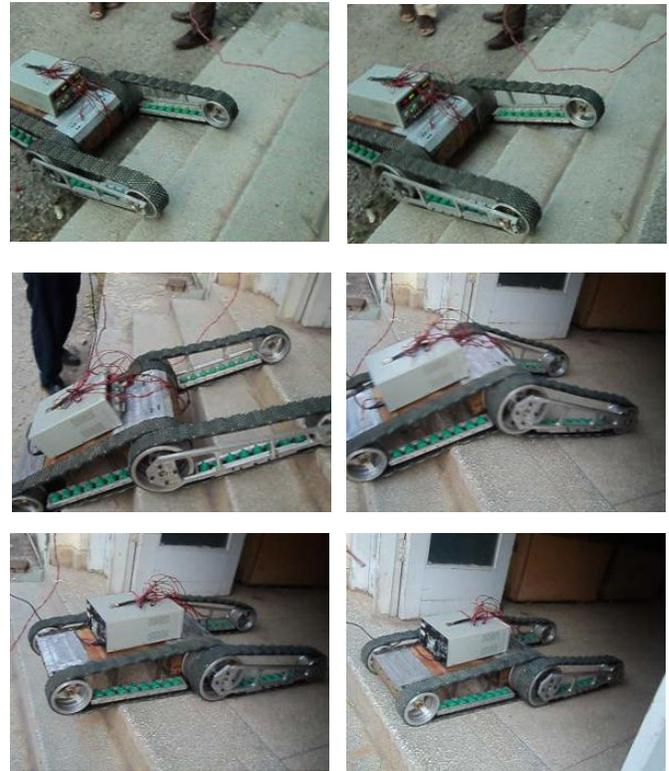
Fig. 10. Actual Robot during Stair Climbing
