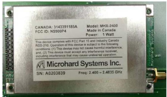
Fig. 2. (b) Microhard MHX-2400 Transceiver [3].
