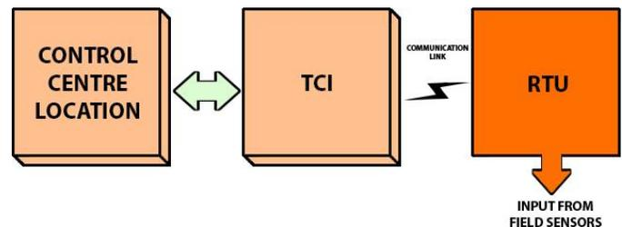
Fig. 1. (a) A general block diagram of Wireless SCADA components including TCI [1].
