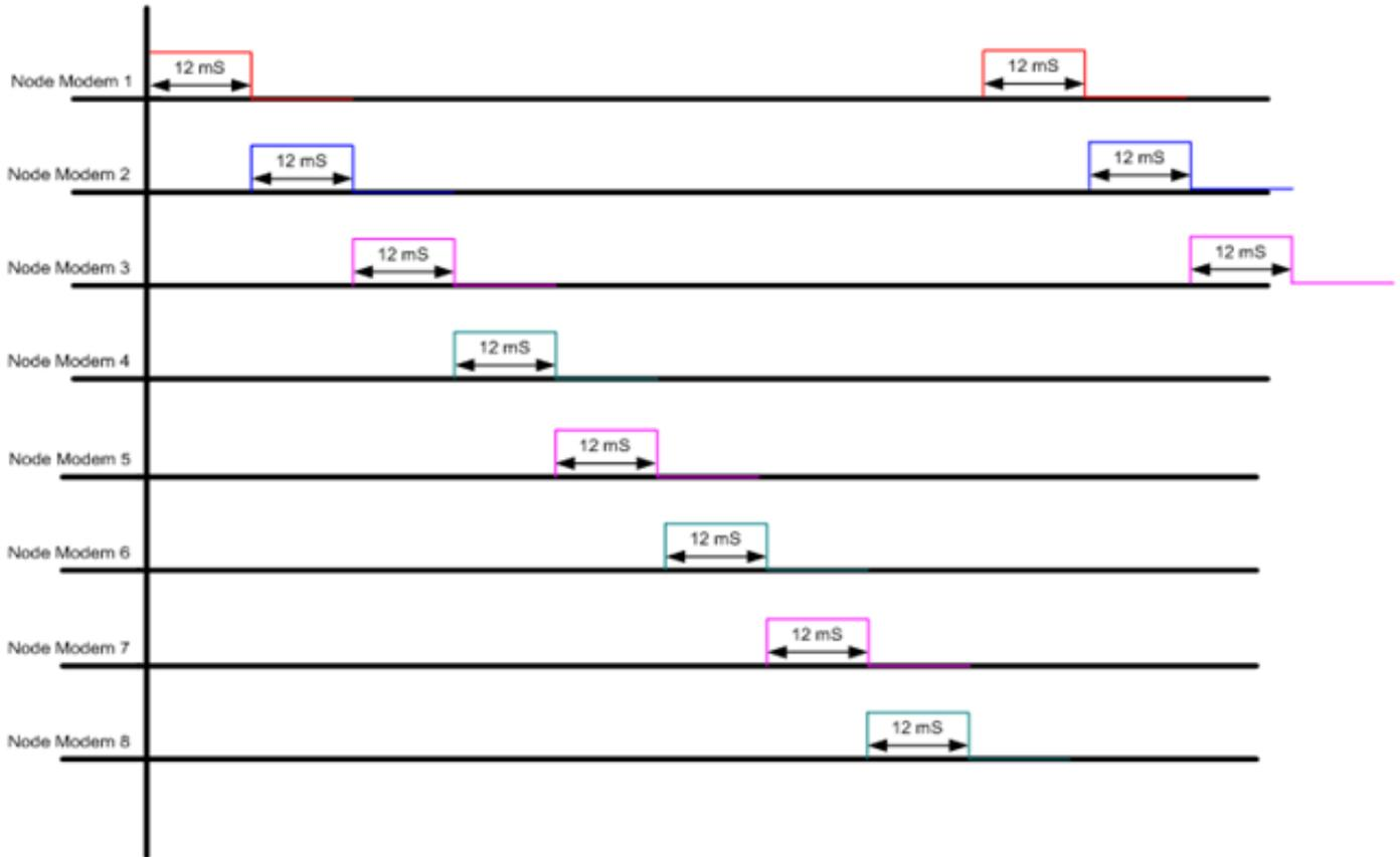
Fig. 3. The Master – Node Communication Timing Diagram.
