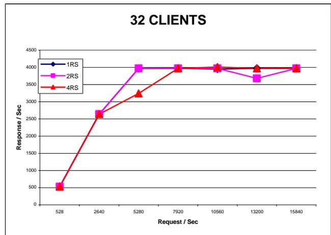
Fig. 9: 32 virtual user with increasing load and different 1, 2 and 4 real server(s)
