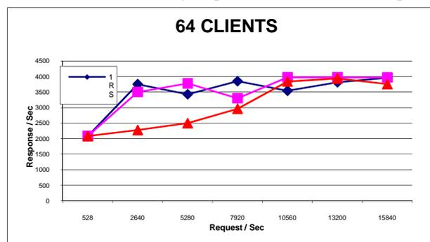
Fig. 10: 64 virtual user with increasing load and different 1, 2 and 4 real server(s)
