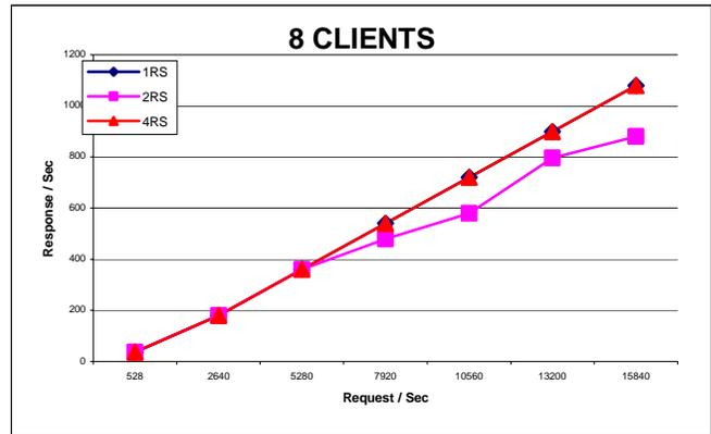
Fig. 7: 8 virtual user with increasing load and different 1, 2 and 4 real server(s)
