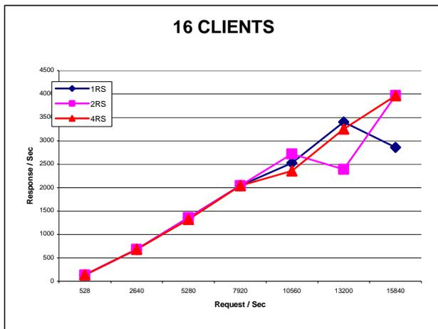
Fig. 8: 16 virtual user with increasing load and different 1, 2 and 4 real server(s)
