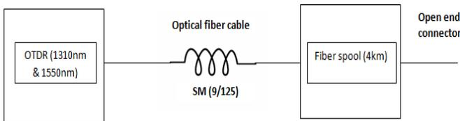
Fig. 3. Attenuation measurements on OTDR
