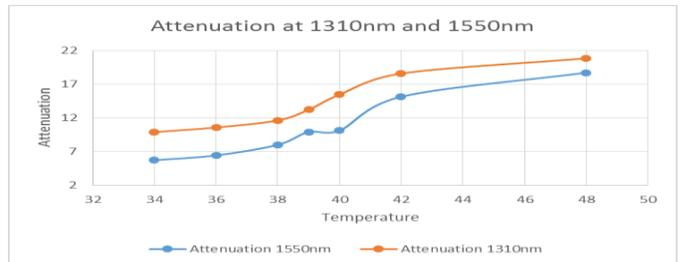
Fig. 12. Comparison graph of Temperature Vs. Attenuation at 4 km
