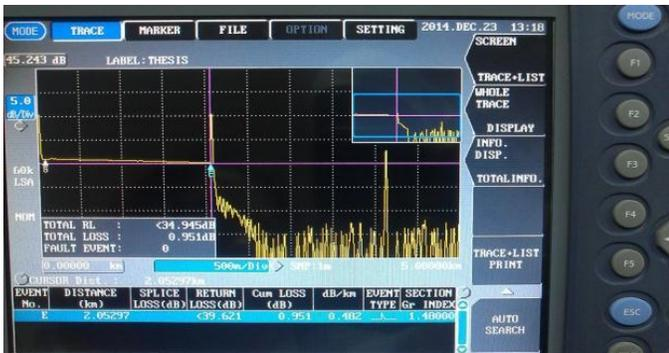
Fig. 7. OTDR analysis at LSA (with stress) 1310 nm
