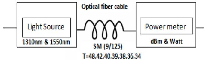
Fig. 4. Power measurements under different temperatures
