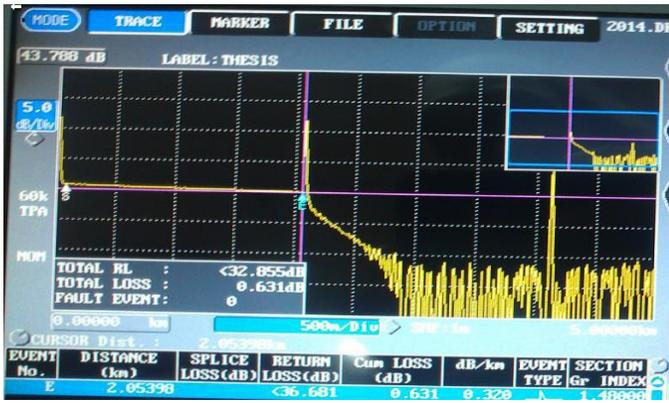
Fig. 10. OTDR analysis at TPA (with stress) 1550 nm
