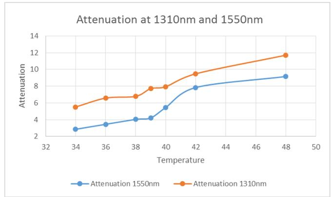
Fig. 11. Comparison graph of Temperature vs. Attenuation at 2 km
