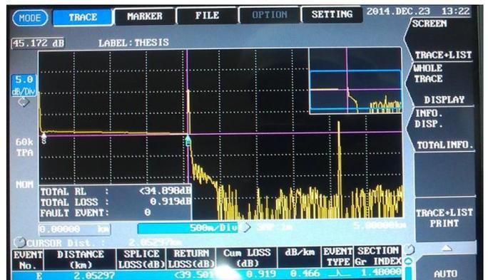
Fig. 9. OTDR analysis at TPA (with stress) 1310 nm
