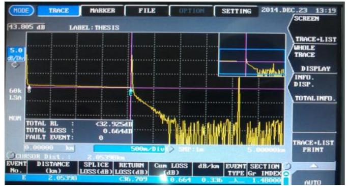
Fig. 8. OTDR analysis at LSA (with stress) 1550 nm
