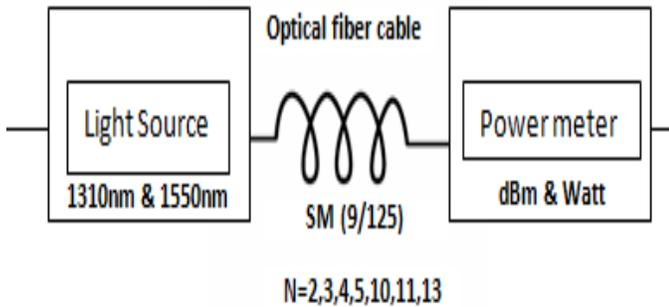
Fig. 2. Power measurements under different bending turns
