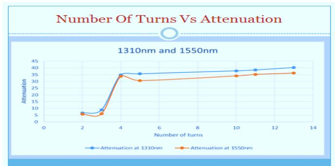
Fig. 6. Comparison of attenuation at different wavelength
