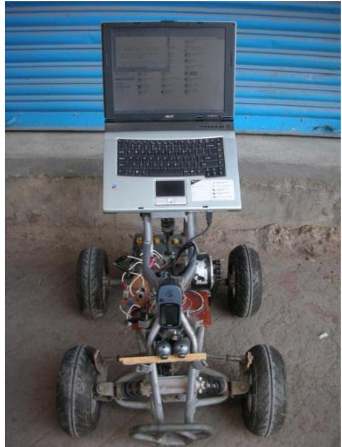
Fig. 1. BMVS for Autonomous Mobile Robot Navigation
